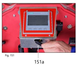
Press the "F3" button (1) on the display and click "next" (2) until page 6 (3) of the menu appears. Unlock the lock (4) with the corresponding access code.
