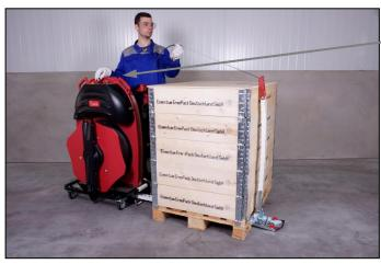
... move the ChainLance completely back by pushing the joystick in "move in" direction.
