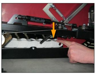
Also for that, the preloaded chain links have to be pressed down with your finger (Fig. 102).
