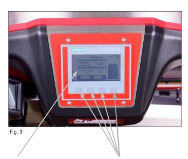
**Touch display** for setting all parameters at the strapping system, such as pallet width.
