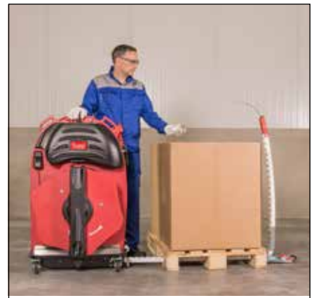
pulls the strap through under the pallet...
