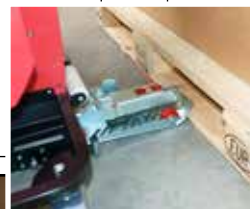
Roll the ErgoPack in front of the pallet. The ChainLance...
