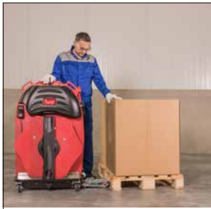
Roll the ErgoPack in front of the pallet. The ChainLance...
