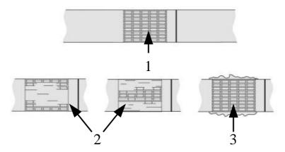
**1 Good welding:** the whole sealed surface has been cleanly welded without any extra material being squeezed out to the side.
