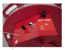
Control with drive unit Cutter Packaging strap brake
