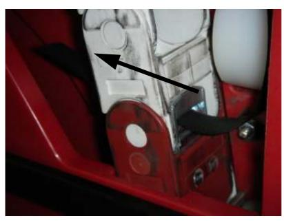
Now close the sliding window (6) Make sure that the window is closed up to the stop. The safety switch for the control unit will only unlock again when the window is completely closed. (red flashing LED turns off, green LED lights up)
