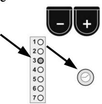
If the necessary welding time is between 6 or 7 to produce a good weld in accordance with point 6.8, or you are unable to achieve a suitable weld using the adjustment methods described above there maybe a fault with the tool or worn component in the welding mechanism. Usually both toothed plates of the welding mechanism have to be replaced.
