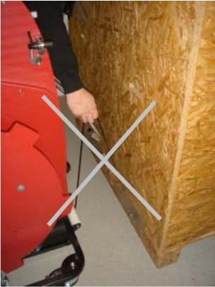
...but about 10 cm below the strap lifter. Hold the strap with the whole hand and pull it out of the unit. <u>You also have</u> to let the end of the strap slide through your other hand at the same time!
