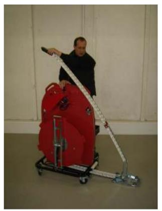
Move the ChainLance out until you are able to place it on the device as shown...
