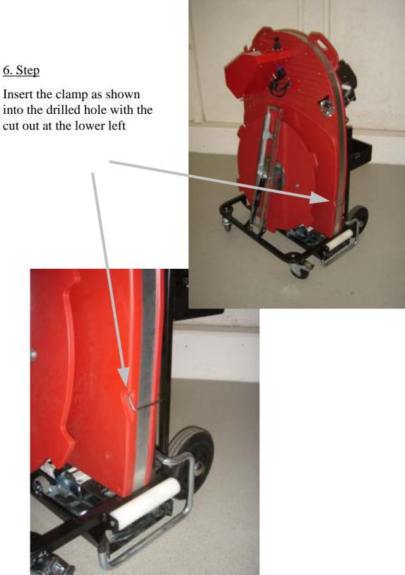
into the drilled hole with the cut out at the lower left
