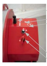
**Joystick** to move "ChainLance" in and out with precision speed control.
