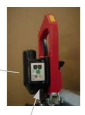
Sealing unit Sliding window with safety switch Tool-Lift Battery
