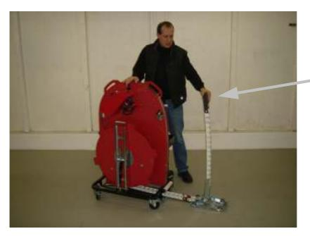
Hold the end of the ChainLance with the left hand while you still continue to push the joystick in the "move out direction".
