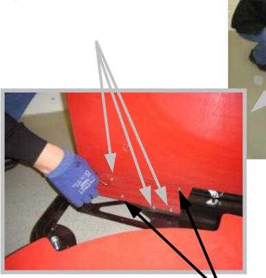
...not the countersunk screws with a 5mm allen key and a 10mm open end or ring spanner on the other side!)
